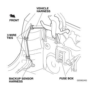
46. Route the backup sensor harness 2-pin connector along the vehicle harness.
