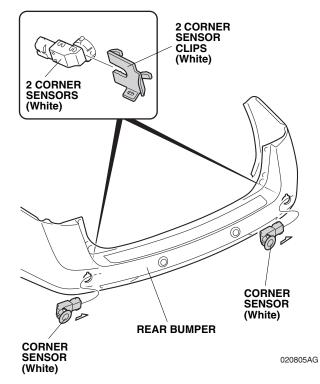
24. Secure two corner sensors (White) with two corner sensor clips (White) as shown.
