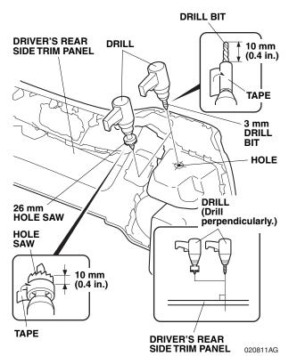
31. From inside of the driver's rear side trim panel, wear eye protection and drill one hole with a 3 mm drill bit.
